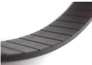
The flat, coated-steel belt eliminates the metal-to-metal effect of conventional systems. Coupled with a smooth-surface crowned machine sheave, the result is exceptionally quiet operation and superior ride comfort. Furthermore, the flexible flat belt enables a more compact, energy-efficient machine, which can be contained in the hoist way. This reduces building and system operating costs and frees up valuable space.
